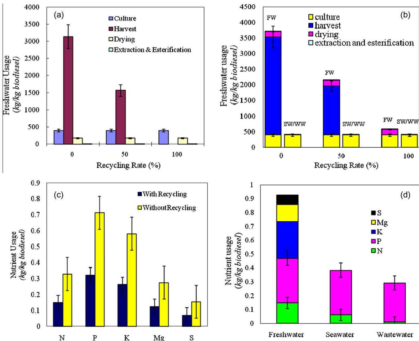
**Fig. 1.** For producing 1 kg biodiesel from microalgae, (a) water footprint using freshwater (FW) medium; (b) water footprint using seawater (SW) or wastewater (WW) as the culture medium; (c) life-cycle usage of nutrients in FW medium with/without harvest water recycling; and (d) life-cycle usage of nutrients in SW or WW medium with 100% harvest water recycling.
