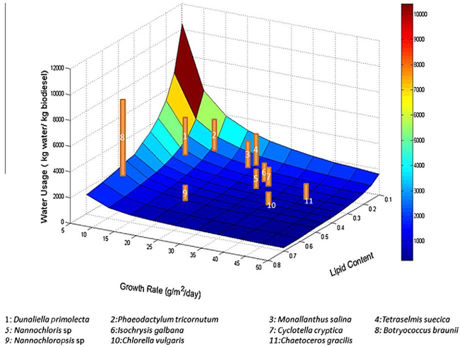
Fig. 3. Water footprint of *C. vulgaris*-based biodiesel production under different algal growth rates and lipid contents. Each bar refers to one reported microalgae species. Details can be found in the electronic annex Table S6.
